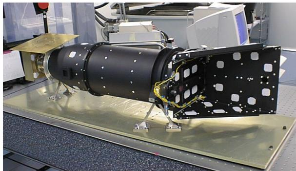
Figure 1. OMC Camera Flight Unit Model during integration and before the installation of the thermal blankets.
