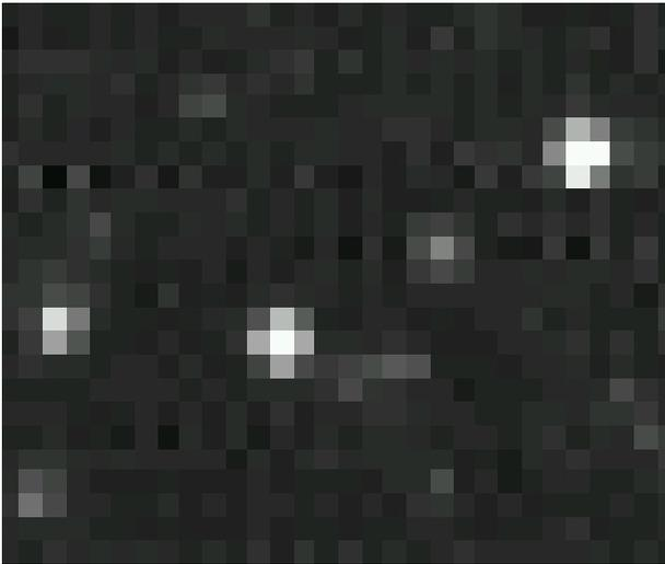
Figure 2. Typical OMC image, showing the Point Spread Function of the system.
