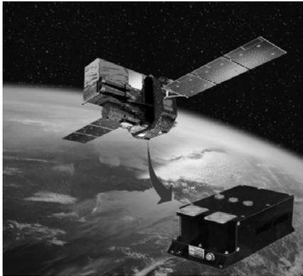
Fig. 5. INTEGRAL with IREM onboard. The end of the arrow shows location of the radiation monitor
